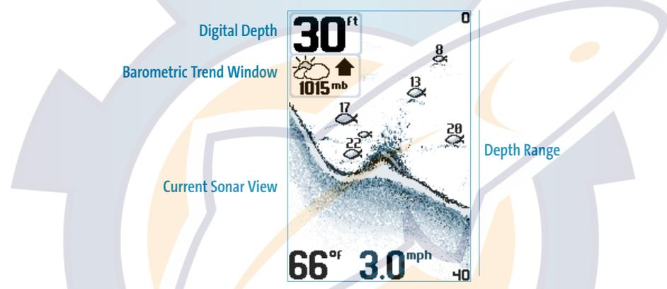
The **WeatherSense View** is automatically added to the Matrix VIEW key list so that it is accessible by pressing the VIEW key. Any of the Matrix views, including WeatherSense, can be removed or added to the rotation list using the Select Views menu (see your Matrix Operation Manual).
